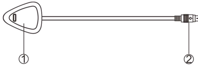
[External window intercom module]
